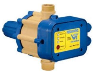
PRESSCONTROL is a device with a new concept that guarantees optimal control of pumps for home use. Deriving from a hydraulic and electronic logics project, it is capable of simultaneously detecting both the pressure and the flow, as well as automatically managing the pump operation.
